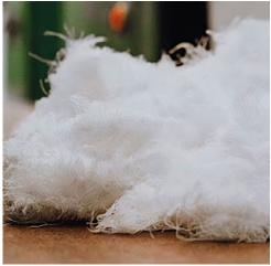
**2. Processing**Using a single-step mechanical process without chemicals, the fibres are garnetted, opened out and recovered.
